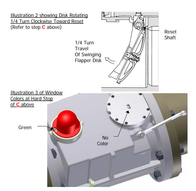
**D**-Release tension on wrench and reset shaft, spring loaded reset shaft will go back to starting position **A**.
